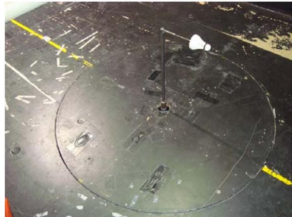
Fig 7d. Complete setup (sting & shuttlecock)
