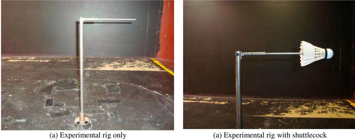
Fig 3. Wind tunnel testing of shuttlecock
