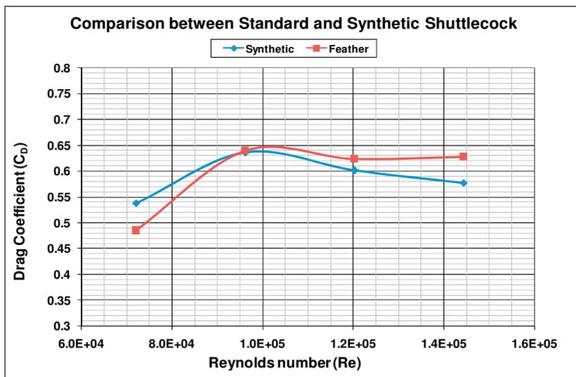
Fig 5. Comparison between Standard feather and Synthetic shuttlecocks
