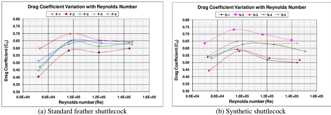
Fig 4.  $C_D$  as a function of Reynolds numbers
